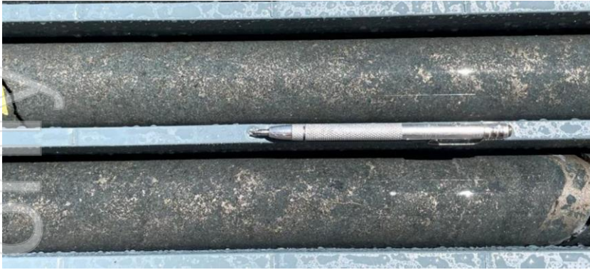
22B2DD003 (40.2-42.0 metres – NQ core 47.6mm diameter) 1.8m @ 2.32% Ni_Eq Strongly mineralised dolerite with disseminated angular blebs of fine-grained pyrrhotite and pentlandite with minor chalcopyrite
